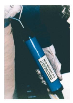
A suction gun that is ideal for use with gear oils to get them both into and out of gearboxes, transfer cases and differentials. Another useful application is to use the C16 suction gun to evacuate the sump of an inboard marine engine.
